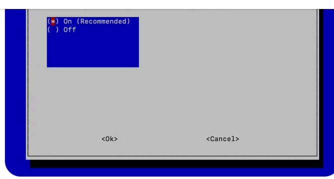
Pi-hole will then ask if you'd like to install the web server. Unless you already have a web server installed that you'd like to integrate with Pi-hole, leave this on as well.
