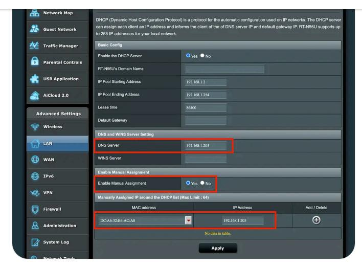
First, enable manual assignment of IP addresses. This is so you can set a static IP address for the Pi that never changes.
