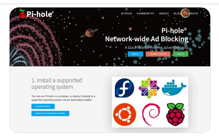
Pi-hole works at the DNS level which means that it intercepts the ads before they're even loaded. It checks every request against a list of known advertisers and if it finds a match, it blocks the request.
